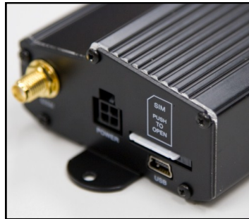
Figure 7. Push in until SIM locks in place
