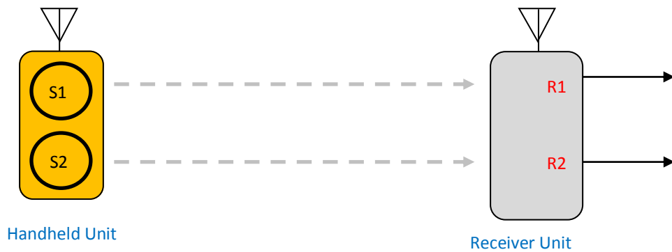
Momentary Function (2 button example): R1 is ON if S1 being pressed, R2 is ON if S2 is being pressed
