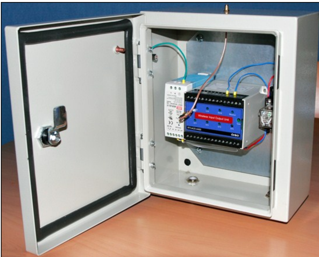
Enclosure showing RTU Module and optional Power supply, External Relay
